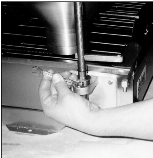
Figure 1-8. Adjusting the Height of the Hopper.
