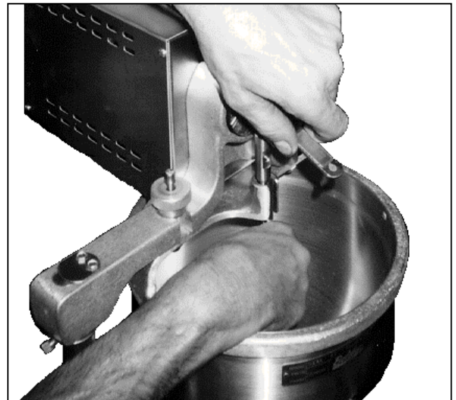
Figure 1-7. Installing the Plunger.
