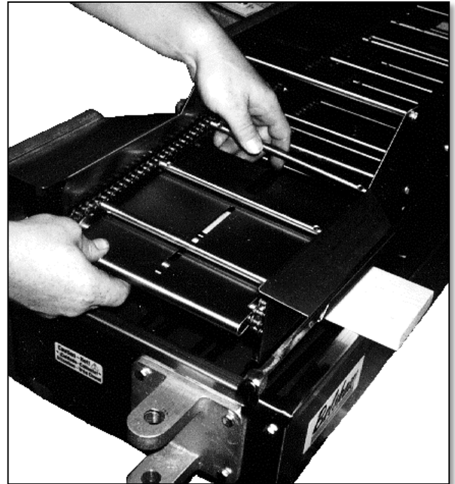
Figure 5 Removing the Drop Plate
